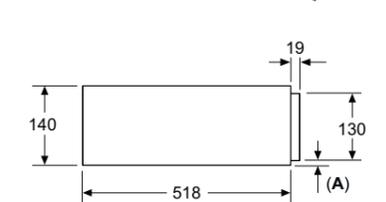
Compact ovens with appliance height of 455 mm can be installed above the warming drawer without an intermediate floor
