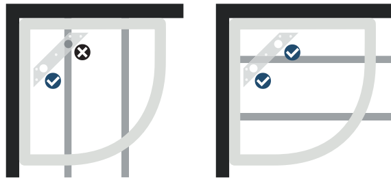
With the unique connect2 design even Quadrant and the Kudos unique Full Curve shape trays have the ability to avoid joists.
